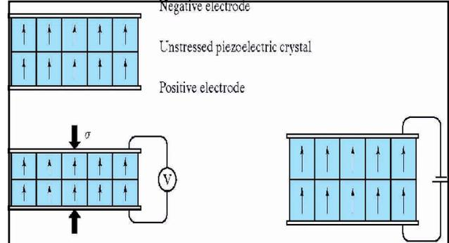
Direct piezoelectric effect      Reverse (converse) piezoelectric effect
