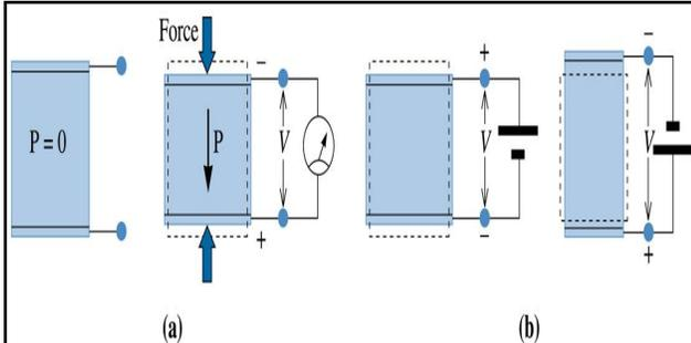
The (a) direct and (b) converse piezoelectric effect. In the direct piezoelectric effect, applied stress causes a voltage to appear. In the converse effect (b), an applied voltage leads to development of strain.
