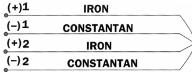
Figure 6. Using a four-wire thermocouple to check for electrical noise picked up in the circuit.
