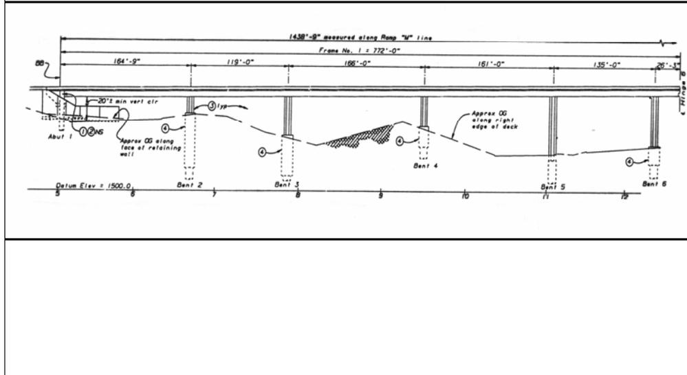
1. Balanced column stiffness is important transversely (previous slide) and longitudinally.
