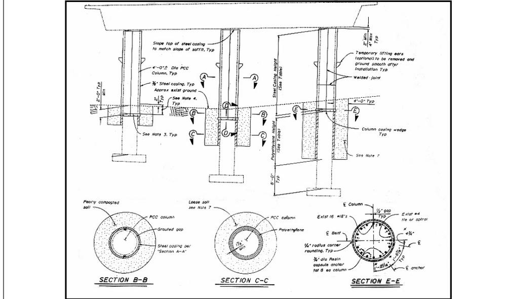
1. Column isolation allows for balance stiffness between columns.
