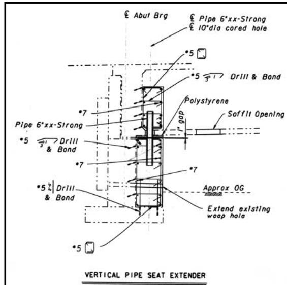
1. This is an abutment retrofit designed to primarily provide lateral (transverse) restraint during a seismic event.
