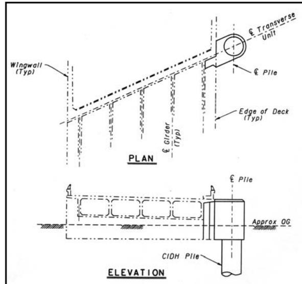
1. This is an abutment foundation retrofit. The pile primarily provides restraint in the transverse direction.
