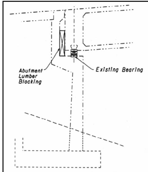
1. This is an abutment retrofit designed to fully engage the soil behind the superstructure.
