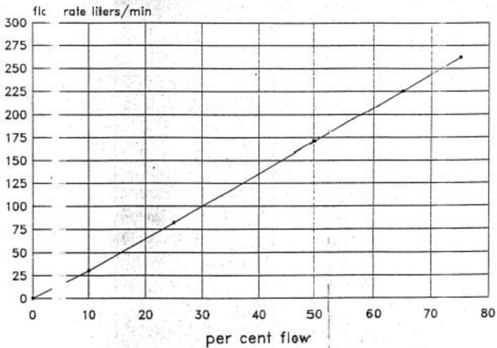
Calibration curves for Rotameter:
