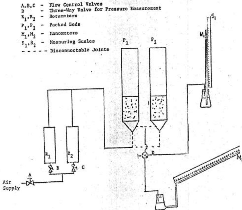
Fig. 1. Flow Sheet for Packed Bed Experiments
