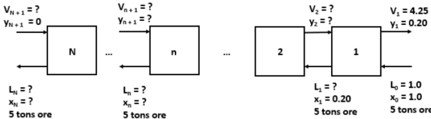
We can choose an arbitrary value for  $x_n$  due to the fact that the stage n is an arbitrary location in the battery.
