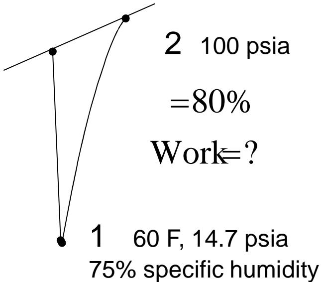
$$T_{2\text{iss}} = T_1 \times e^{\left( \frac{(R_{\text{air}} + c_p R_{\text{vapor}})}{(c_p \text{pair} + c_p \text{vapor})} \ln \left( \frac{p_2}{p_1} \right) \right)}$$
