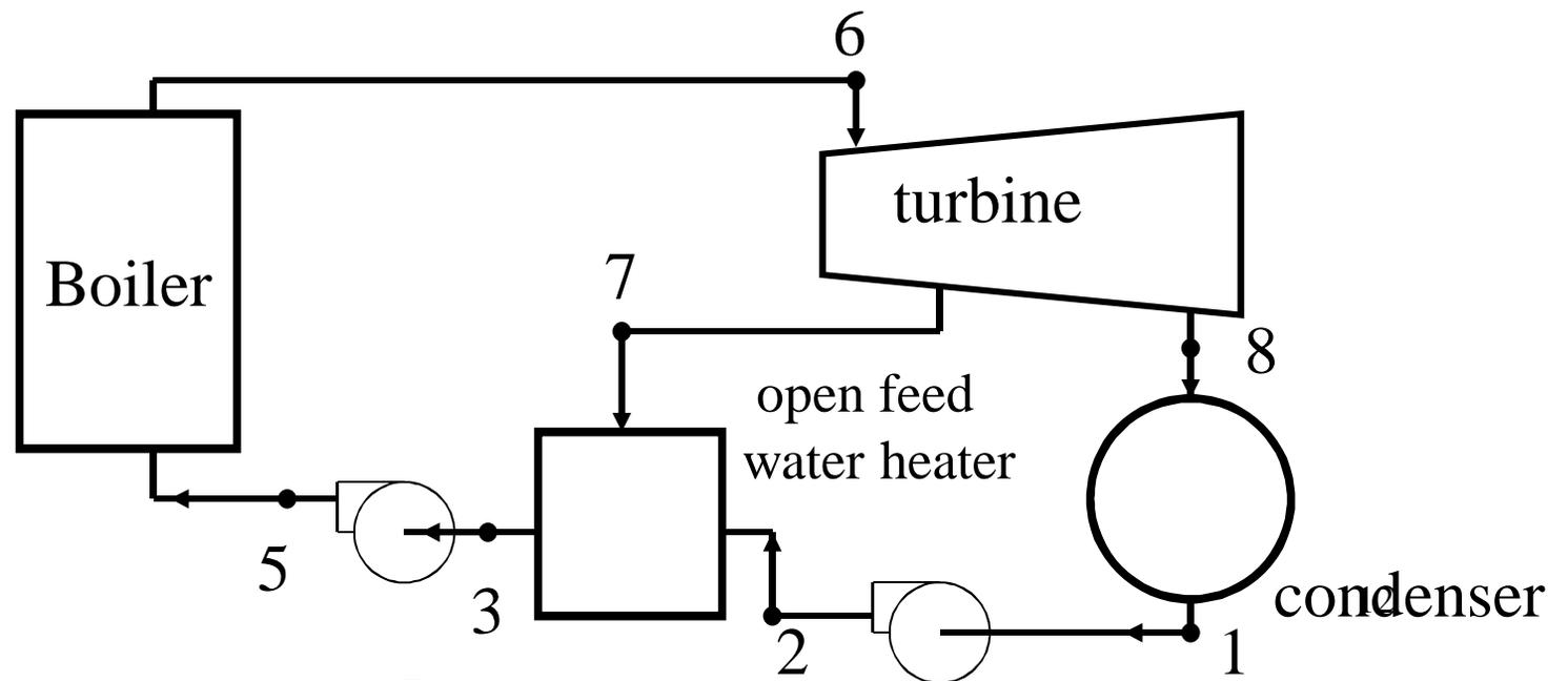
**A steam power plant runs on a regenerative cycle and produces 80 MW. The turbine inlet conditions are 10 MPA, 550 C. Steam is extracted at .8 MPA to feed an open feed water heater the rest is reheated to 500 C. The condenser operates at 10 kPa.**
