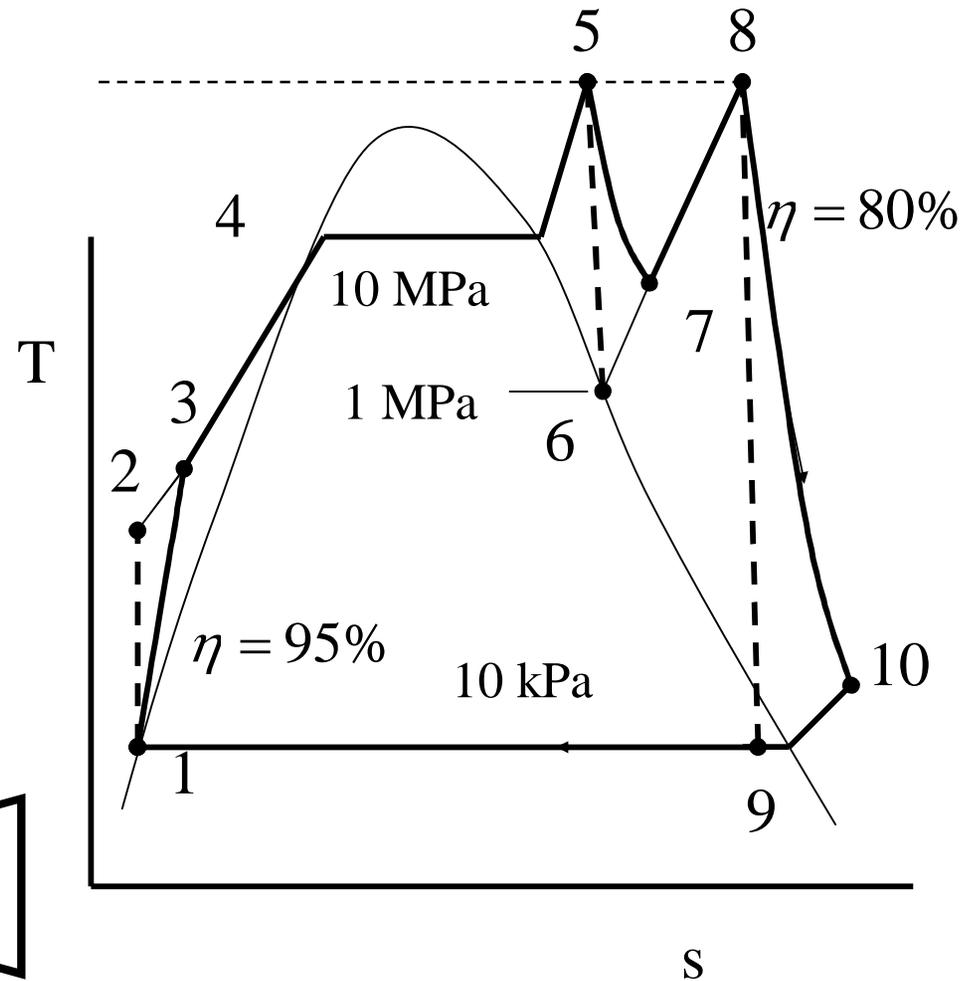
A steam power plant runs on a reheat cycle and produces 80 MW. The turbine inlet conditions are 10 MPa, 500 C and 1 MPa, 500 C. The condenser operates at 10 kPa. The efficiency of the turbines is 80%. The efficiency of the pump is 95%. Determine: a) the turbine exit conditions, b) the cycle efficiency and c) the mass flow rate of the steam.
