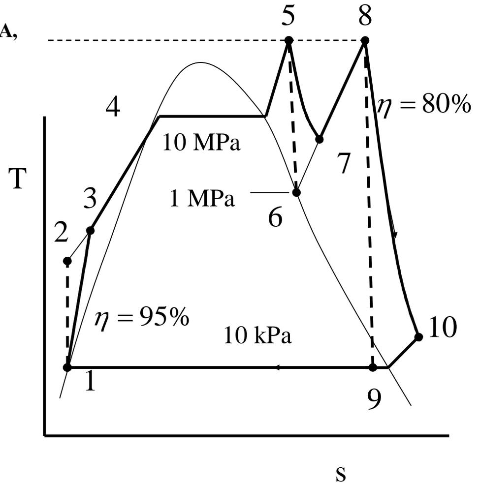
compressed liquid water, Table A - 7,  $p_2 = 10\text{MPa}$
