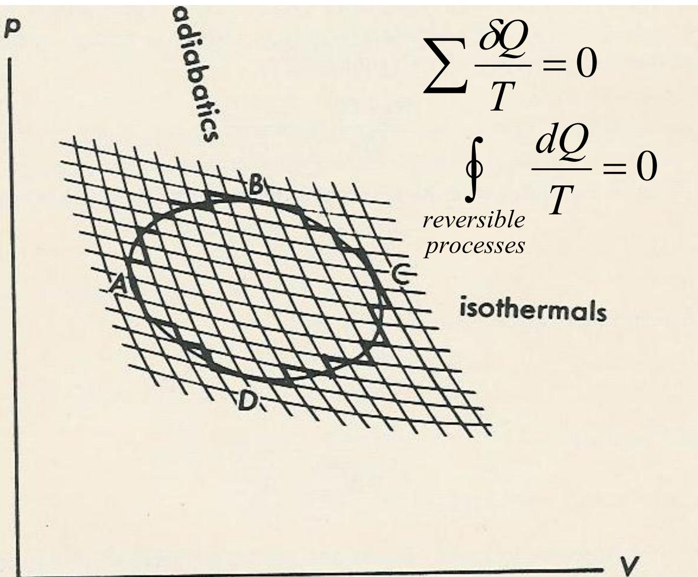
Fig. 9.2 General Cycle Approximated by Large Number of Carnot Cycles.
