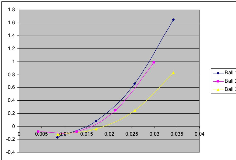
The principal effects of roughness seem to be to decrease the lift coefficient at high spin rates. Note also the negative lift coefficients at low spin rates. This spin reversal is seen in experiments but it is not well understood. It seems likely to be a low Reynolds number phenomenon. We have not considered Reynolds number in plotting these data, so that these effects are not known from this data.
