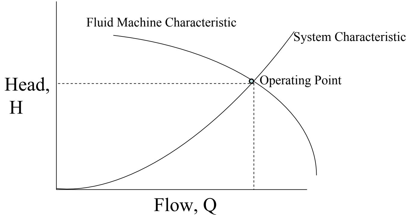
Energy (head) is put into the system fluid by the fluid machine in the form of velocity and pressure.
