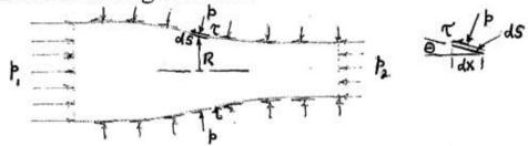
Average pressure =  $\int pdA = \overline{p}A$  on entrance and exit areas Forces from duct wall:
