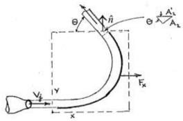
Neglect friction effects, the vane simply turns the fluid while the speed of the fluid is constant
