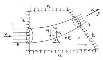
Weight of the pipe bend =  $W_b$ Weight of the fluid in the bend =  $W_f$ .
