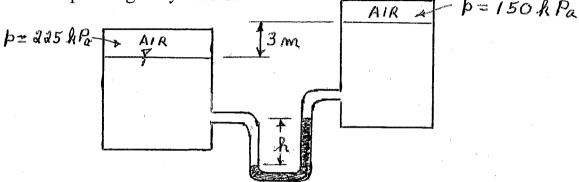
2.2 The tank holds water, oil (s.g. = 0.7), and air as shown. What is the pressure in the air?
