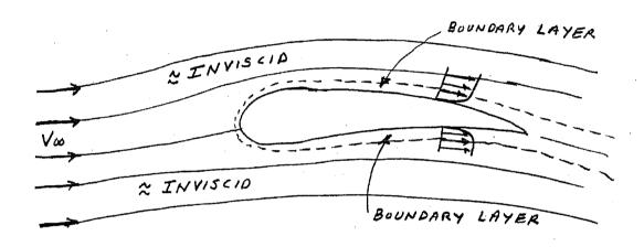
Since the boundary layer is relatively thin, it does not significantly affect the flow outside the boundary layer which can be considered inviscid.
