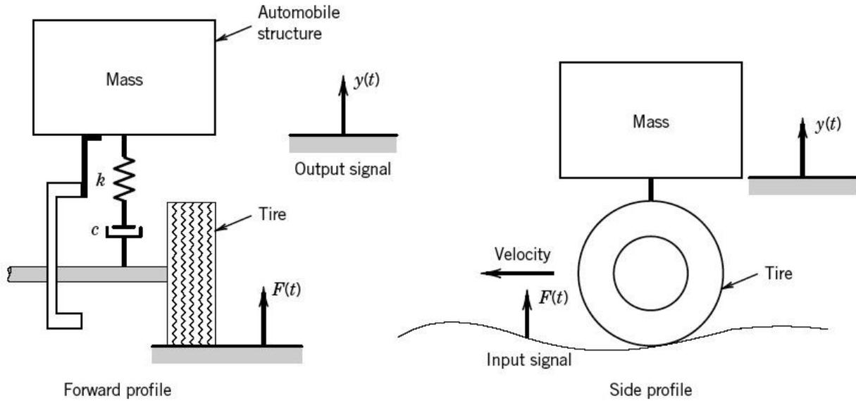
**Figure 3.1** Model of an automobile suspension with input and output signals.
