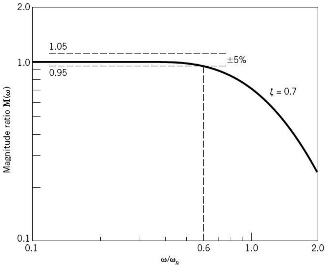
**Figure 3.18** Magnitude ratio for second-order system with  $\zeta = 0.7$  for Example 3.10.
