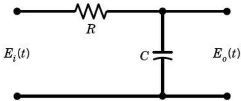
Figure 6.29 Low-pass RC Butterworth filter circuit.
