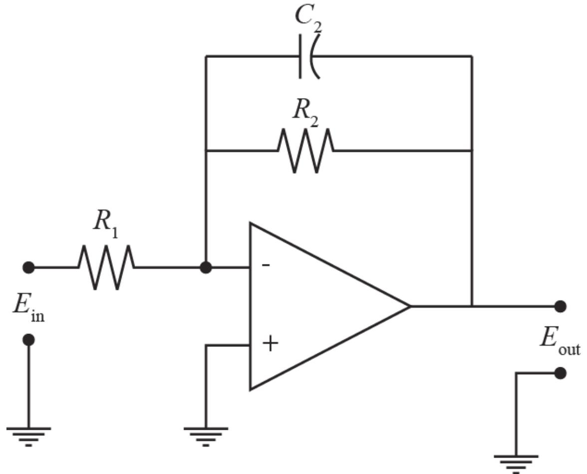
22. The static sensitivity of the amplifier circuit is  $R_2/R_1$ .
