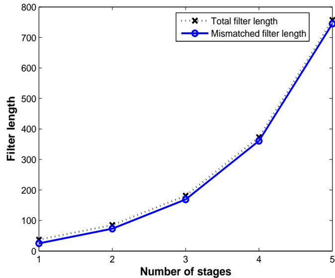
**Fig. 5.** Filter lengths as functions of the number of stages
