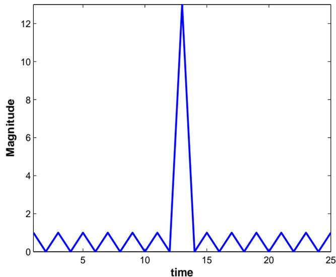
**Fig. 2.** Output of the matched filter
