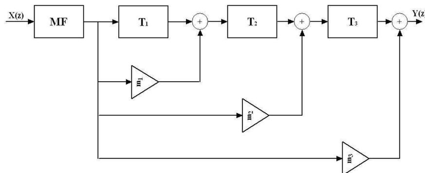
**Fig. 1.** Structure of the proposed filter
