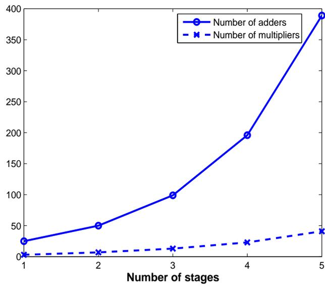
**Fig. 6.** Number of adders and multipliers required for different number of stages
