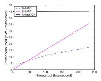
Figure 8: The measured power consumption of maintaining a given throughput in a 10-node network. As the throughput increases, the overhead of S-MAC's SYNC period causes the power consumption to increase linearly. The throughput is the average node bitrate (number of data bytes sent in a 10 second time period) in the 10 node network.
