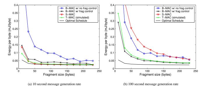
Figure 9: The effective energy consumption per byte at node C for a network as shown in Figure 10. Each node generates a message every 10 seconds (left) and every 100 seconds (right) consisting of 10 fragments of the size given on the x-axis.
