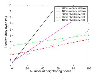
Figure 5: The node's duty cycle is affected by the network density and LPL check interval. Typically used LPL check intervals in B-MAC's implementation are depicted. The best check interval is the lowest line at a given network density.
