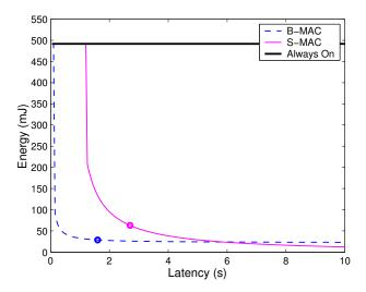
Figure 12: As the latency increases, the energy consumed by both B-MAC and S-MAC decreases. The point illustrated on the B-MAC line is the default configuration as shown in Table 3. The point on the S-MAC line is the default S-MAC configuration at 10% duty cycle with adaptive listening.
