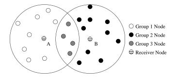
Fig. 11. Group TDMA Receiver-Based Grouping
