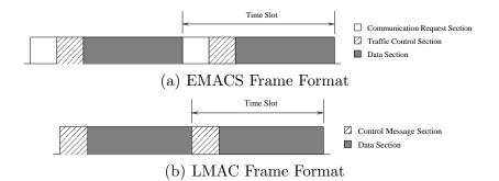
Fig. 13. EMACS and LMAC Frame Formats
