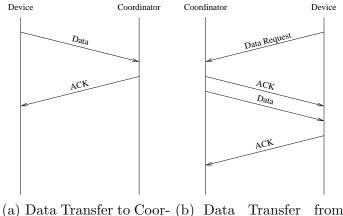
(a) Data Transfer to Coor- (b) Data Transfer from dinator Coordinator
