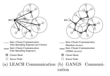
Fig. 10. LEACH and GANGS Communication Comparison
