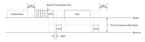
Fig. 2. IEEE 802.11 DCF Backoff Algorithm and Message Transfer
