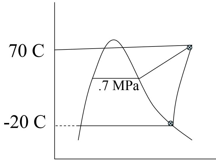
$$@ -20^{\circ}\text{C}, v_g = .146 \text{ m}^3/\text{kg}, h_g = 235.3 \text{ kJ/kg}$$
