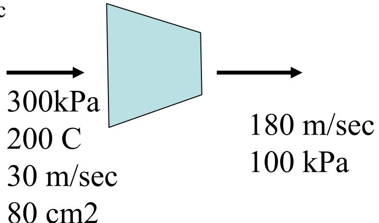
$$v_2 = \frac{RT_2}{p_2} = \frac{.287 \times (273.15 + 184.5)}{100 \text{ kPa}}$$
