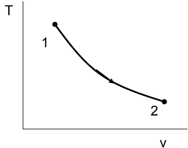
$$p_2 = p_1 \left( \frac{v_1}{v_2} \right)^2 = 500 \left( \frac{1.701}{3.8} \right)^2 = 100 \text{ psi}$$
