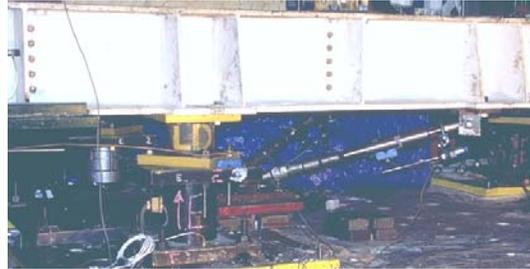
SHAKE TABLE TESTING OF SEISMICALLY ISOLATED STRUCTURE WITH HYBRID SYSTEMS AT UNIV. AT BUFFALO
