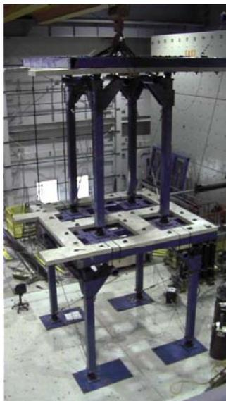
**Modular and versatile two-level platform for experimental seismic performance evaluation of full-scale nonstructural components, systems and equipment under realistic full-scale building floor motions**
