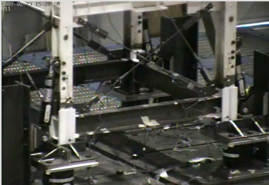
Synthetic EQ 175% of Design - Viscous Dampers
