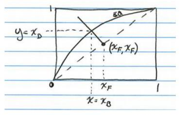
Now that you have (x, y), you can determine the Flash temperature on the T<sub>xy</sub> diagram
